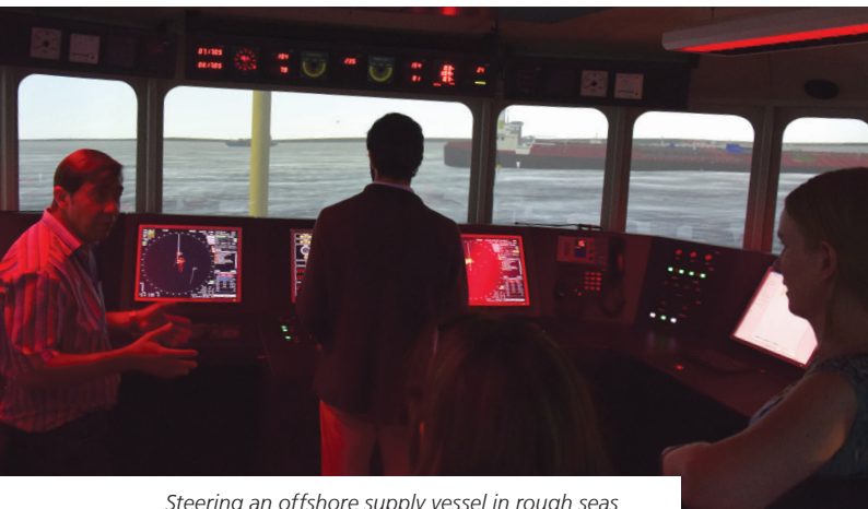
Steering an offshore supply vessel in rough seas using the bridge simulator at Force Technology.
